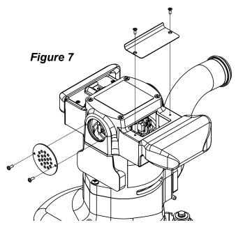
CAUTION: Use only motor brush PN 40818A or PN 40055A with shunt wire or motor failure will occur.
