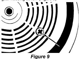
Align the holes with each of the other two screws, then remove screws.
